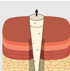
**2** Gently pull the plug partially out of the internal opening.
